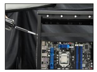
4. Place the SOLO II on its side. Position the PSU into the mount and secure it with the PSU screws provided. If your PSU has a fan on its top side, make sure it aligns with the SOLO II's top intake vent.
